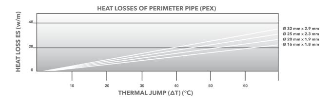
In general, we can conclude that its Low thermal conductivity coefficient (0.38 W/mK) provides energy saving by reducing losses of heat. Consequence of its low coefficient of thermal conductivity is that the usual condensations of metal pipes are rare in the cross-linked polyethylene Astral PEX-a Pro piping.
