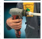
(\*) this turning of the expansion head is only necessary while using manual expanders without rotating expanding heads (for expanders equipped with rotating expansion heads, this turning of the expansion heads is not necessary).
