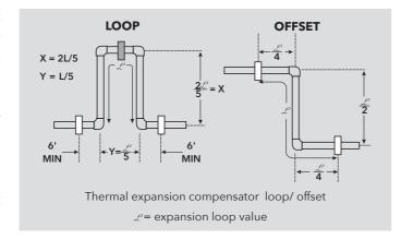
For convenience, loop (or offset) length have been calculated for different pipe sizes and different run length with a temperature. The results, shown in tables, are presented simply as handy guide for quick and easy determinations of acceptable loop length for the approximate conditions. Loop length for other temperatures and run length can be kept as per given table herewith:
