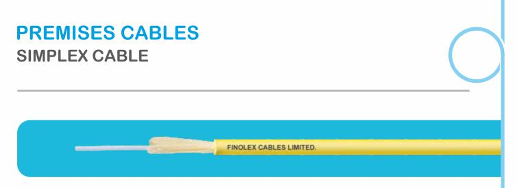
1 Fibre Tight Coated With PVC Or Lszh Is Placed In Lszh Sheath With Aramid Yarn. Optical Fibre Used Is Bending Loss Insensitive which is Suitable in FTTH Network For Indoor Application.
